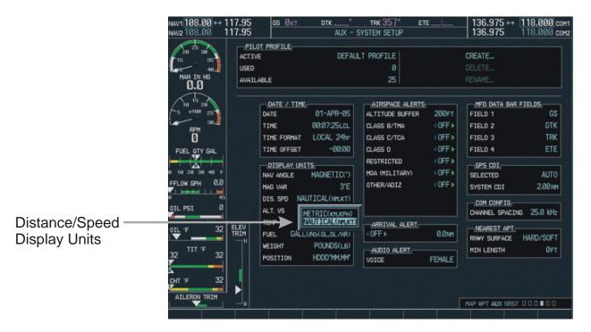
Figure 2. AUX-System Setup Page Distance/Speed Setting
