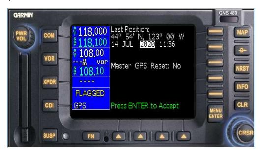
4. Once the correct date is entered, use the outer and inner cursor knobs to set Master GPS Reset to YES.
