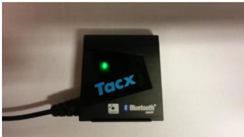
The unit has a built-in flashing green light, that will go on every 15 seconds. It is activated the moment the magnet is passing the cadence sensor or the speed sensor. In the T2015 there are 2 sensors built in.
